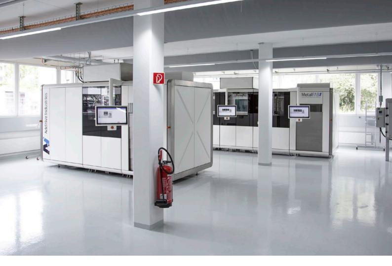
Today, Sauber Engineering houses 13 large-format polymer 3D printing systems, four MetalFAB1 printers and an HIP system. Image: Sauber Motorsport AG
