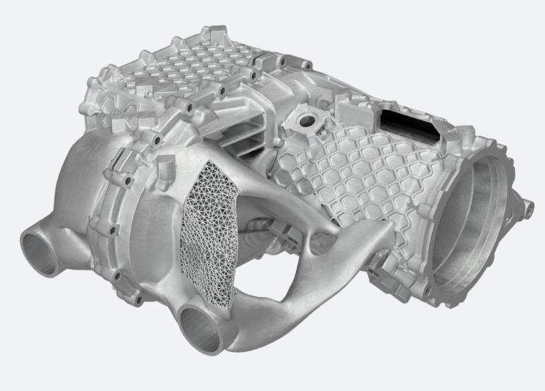
Porsche and SLM Solutions developed a E-Drive housing using the latter's 12-laser NXG XII 600 PBF system. Image: Porsche AG
